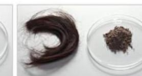
▲ Before and after grinding of hair samples using LAWSON grinding apparatus
