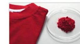
▲ Lapping analysis of fiber sample with KBr particles
